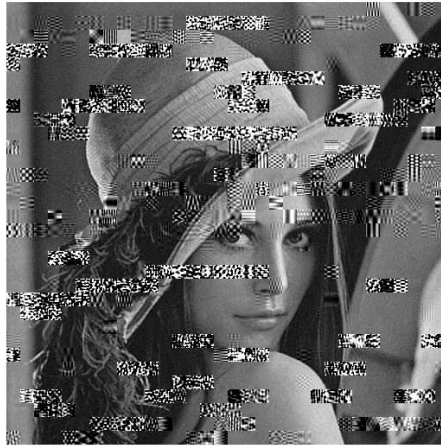
Figure 15: Received picture sent from our TX PCB and received with an advanced RX2400 board with a distance of roughly 40cm.
