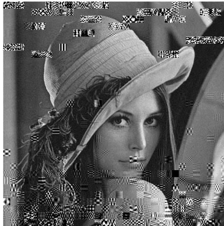
Figure 16: Received picture sent from an advanced RX2400 board and received by our receiver PCB with a distance 1m.
