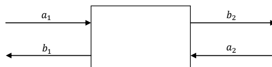
Figure 2.1: The common 2-port. Incident waves are represented by a_1 and a_2 . In the same manner outgoing waves are represented by b_1 and b_2 .
