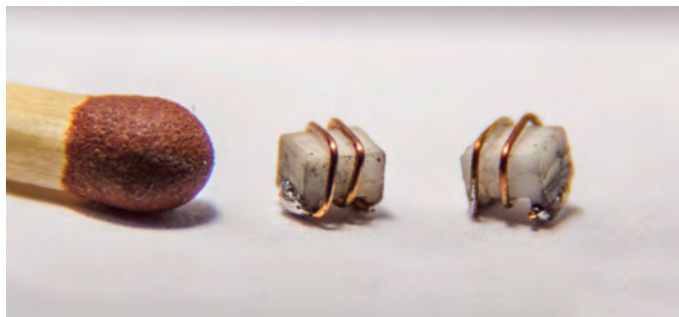
Figure 3.44: The final design of the drain bias inductors shown together with the head of a match. The thickness of the copper wire used is 0.25 mm.
